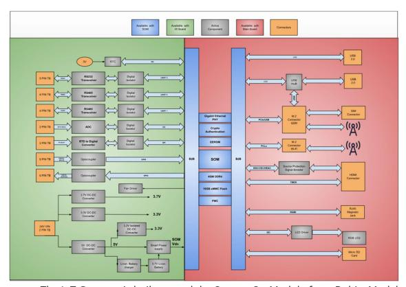
The IoT Gateway is built around the System On Module from Debix. Model number Debix SOM A. The SoC i.MX 8M-Plus on SOM supports both Linux and Windows IoT OS. The IoT Gateway unit comprises of two PCBAs named as Main Board and I/O Board, where baseboard connects with the SOM module using 4
